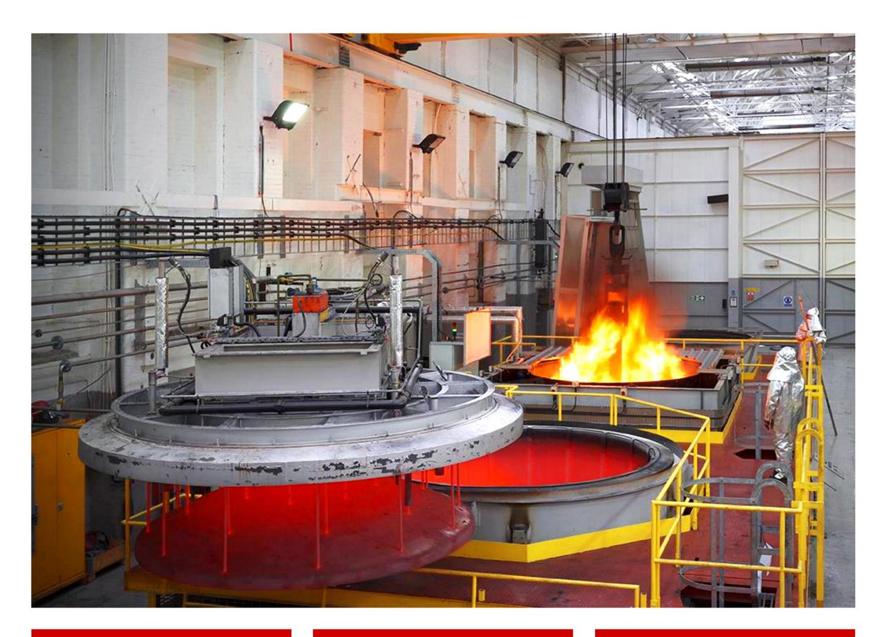
Rated temperature 950°C ~ 1200°C Rated Power 60 ~ 1500Kw
